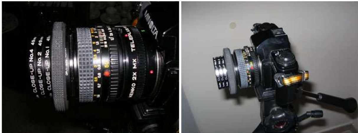
FIG. 2: USE OF ADDITIONAL LENSES; THE MOST ECONOMIC SYSTEM FOR THE MACROPHOTOGRAPHY
